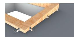
Screw the brackets into the roof/kerb approximately 100mm from each corner and centres of the kerb. More for larger kerbs - approx every metre. The brackets must be screwed through structural elements, not the insulation, to get a firm fix.
