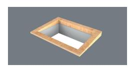
4) Make sure you have the 'fall' in the correct direction. Place the kerb over the prepared aperture and align. Push the rooflight kerb down nice and tight. If some silicone bleeds out just wipe it clean. The upstand/kerb must sit flat. If uneven, use packers where required.
