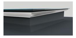
**10)** Affix the roof covering up the side of the kerb/frame and under the 15mm gap between the main box section frame and the curved external section. If using a torch to heat the roof covering material, only heat the roof covering before affixing.
